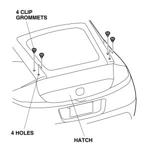
15. Install the four pins onto the hatch spoiler.
