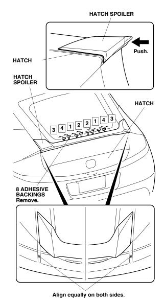
20. Using the palm of your hand, firmly press the hatch spoiler to the hatch for 30 seconds.
